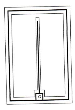
Top Material: Al Backside Material: Ti/Ni/AG Bond Pad Size: .020" X .020" Backside Potential: Drain Mask Ref: M000348A
